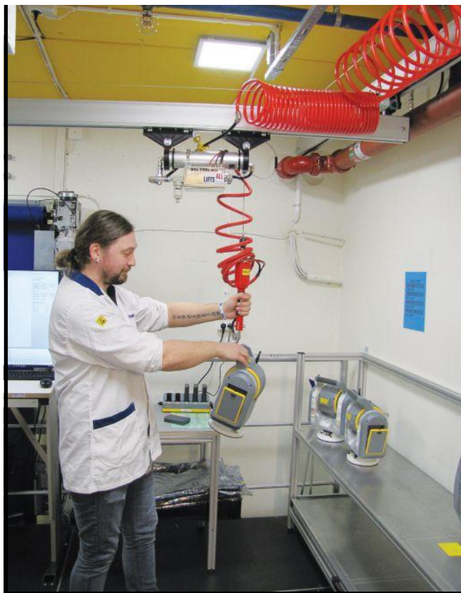
Manufacturing technician Maik Tegge demonstrates how the SX10 is being hoisted into climate-controlled chambers for testing from -20°C to +50°C.
