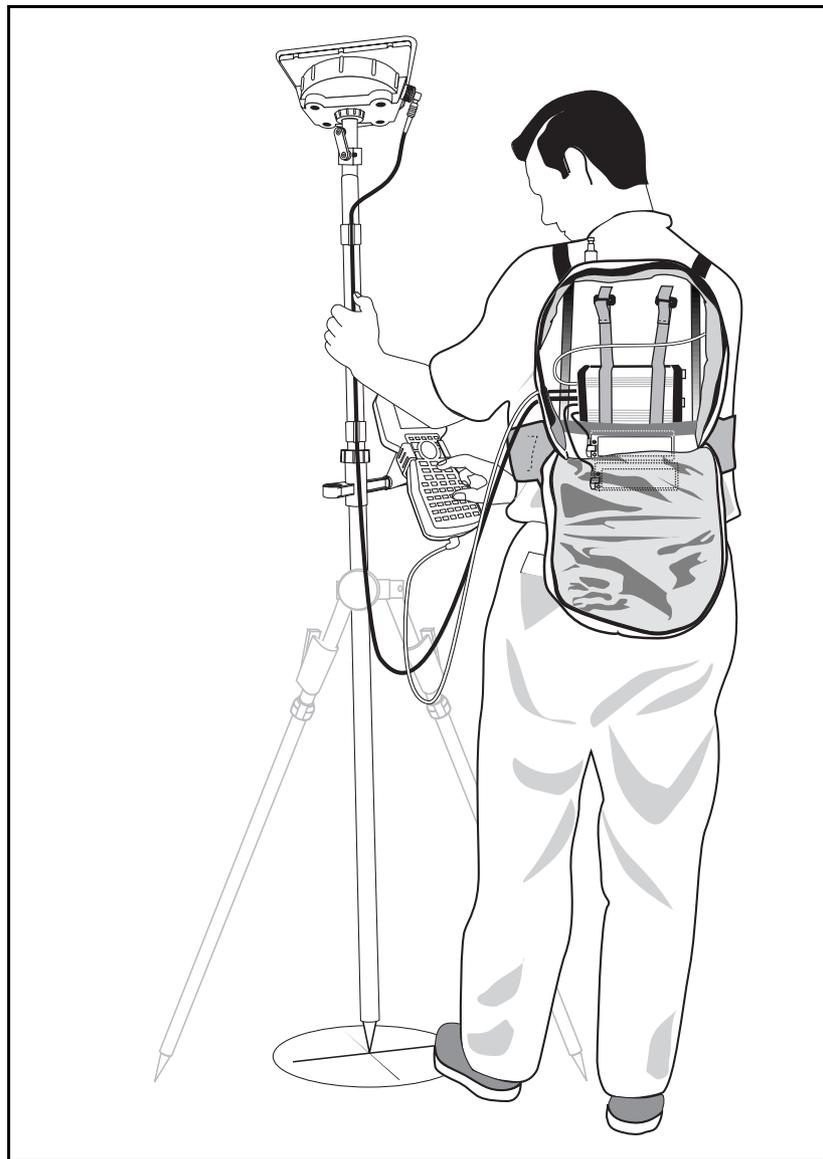
**Figure 4-4 Using a Rangepole With the 4700 Receiver**
