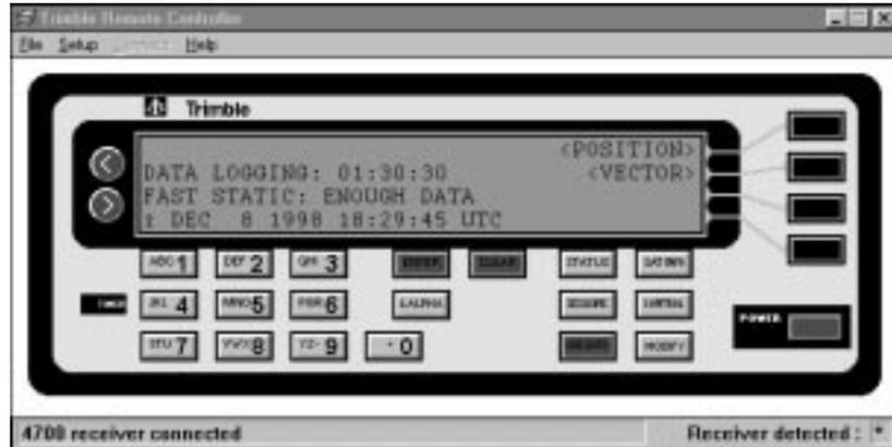
**Figure E-1 Simulated 4700 Receiver Front Panel**
