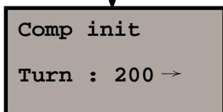
Turn the instrument back 200 gon(180°) and the display will automatically change to.....
