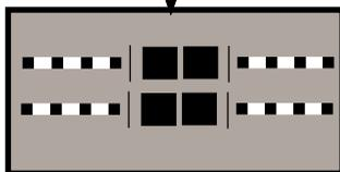
.....display of the electronic level which indicates the level status of both axes of the instrument. As no measurements are to be made we will disconnect the dual axis compensator with function No. 22. Press F22 ENT.
