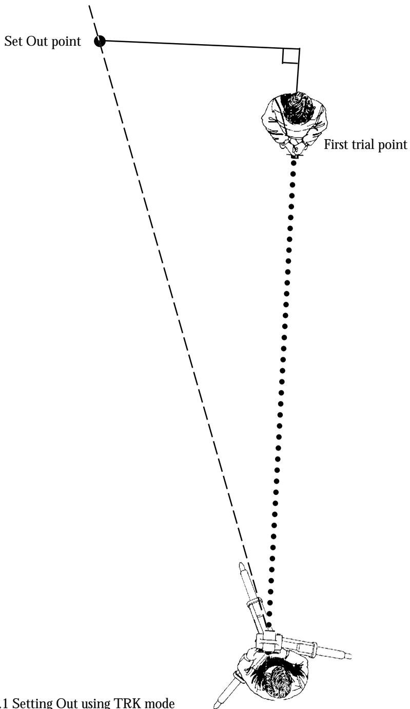
Fig 4.1 Setting Out using TRK mode
