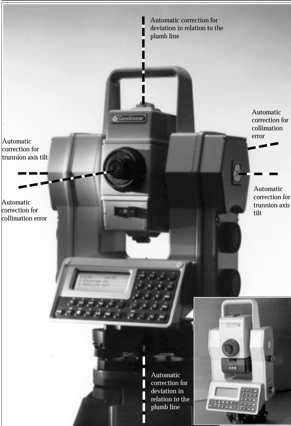
Fig 1.1 The Angle Measurement System
