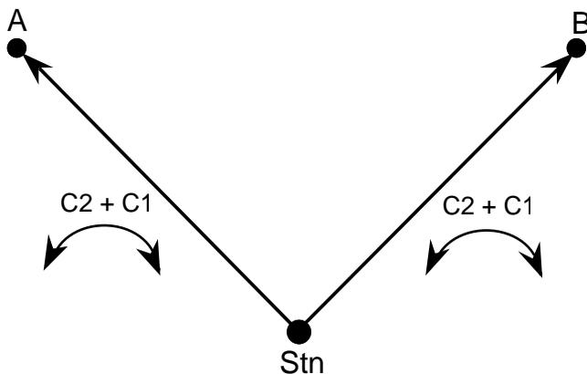
Fig. 1.2 Two-Face Angle Measurement.
