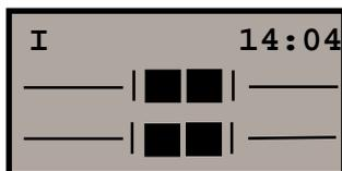
The instrument is levelled.
