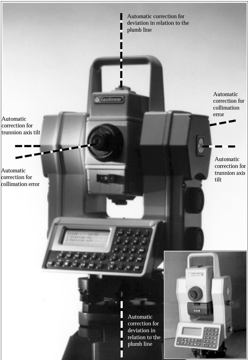
Fig 1.1 The Angle Measurement System
