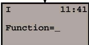
Key in the label number for instrument height, 3 and press the ENT-key.
