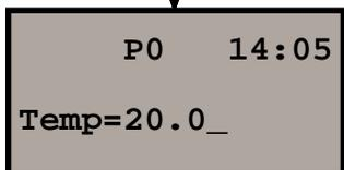
.....program 0. The appearance of P0 indicates that the instrument is sufficiently well levelled and that the compensator is now engaged. It also means that the electronic level is in the "fine mode" in which each individual left or right movement of the cursor represents 20 °C.
