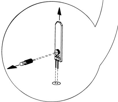
Fig 3.5 The sketch shows how the Tracklight bulb ( 6.3V /0.2A) should be removed from the connection socket.
