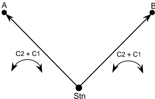
Fig. 1.2 Two-Face Angle Measurement.
