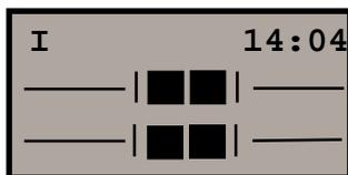
The instrument is levelled.
