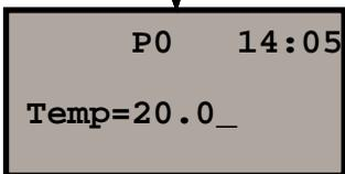
.....program 0. The appearance of PO indicates that the instrument is sufficiently well levelled and that the compensator is now engaged. It also means that the electronic level is in the "fine mode" in which each individual left or right movement of the cursor represents 20<sup>CC</sup>
