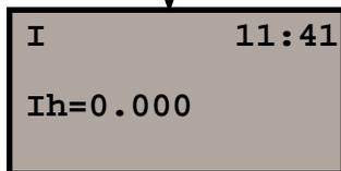
*The display shows the current value for the instrument height
