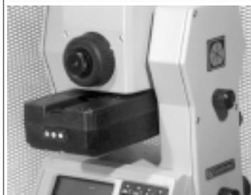
Fig. 2.1 Connecting the internal battery
