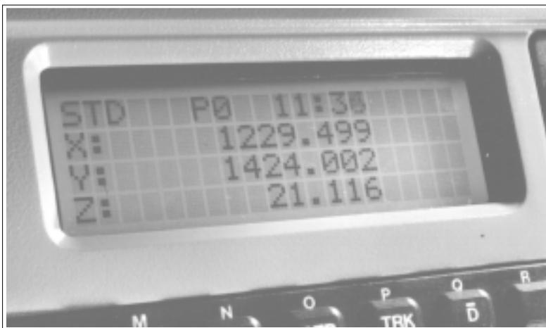
Fig. 1.4 Display with alphanumeric keyboard
