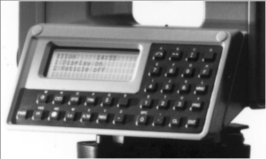
Fig 1.5 Geodimeter with alphanumeric keyboard
