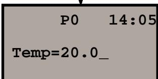
.....program 0. The apperance of PO indicates that the instrument is sufficiently well levelled and that the compensator is now engaged. It also means that the electronic level is in the "fine mode" in which each individual left or right movement of the cursor represents 20<sup>CC</sup>
