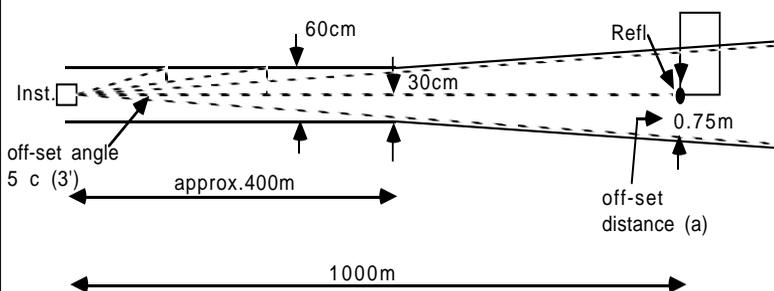
Fig. 2.1 Measurement towards an eccentric point.
