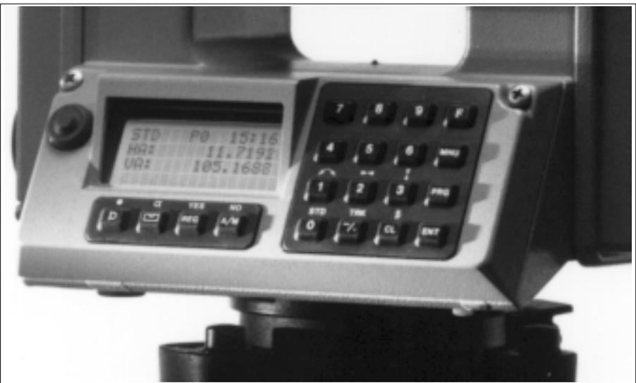
Fig 1.6 Geodimeter with numeric keyboard
