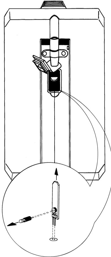
Fig 3.6 The sketch shows how the Tracklight bulb ( 6.3V /0.2A) should be removed from the connection socket.
