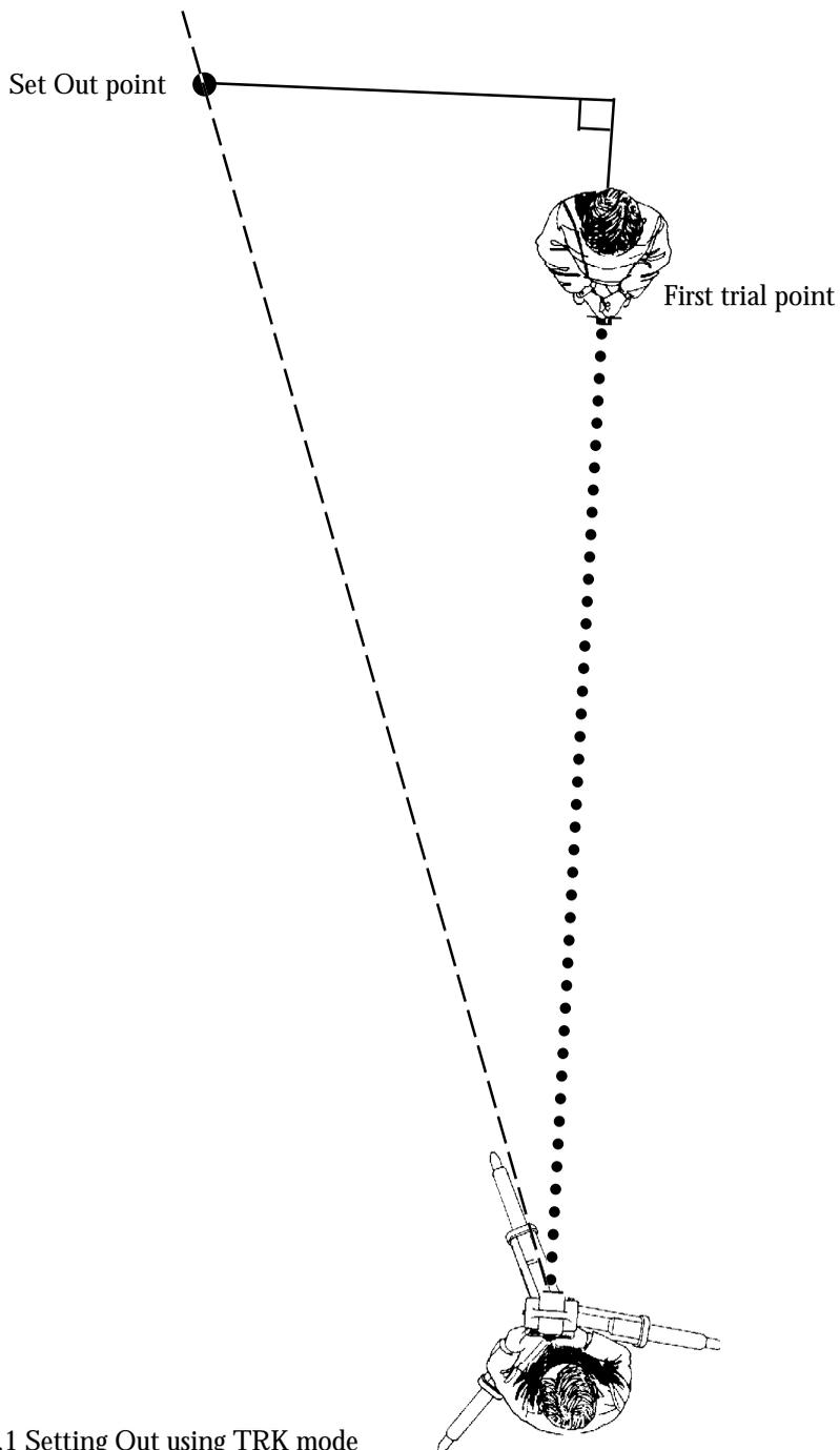
Fig 4.1 Setting Out using TRK mode
