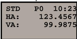
After answering Yes to storage of the horizontal axis tilt correction factor, you are automatically returned to the P0 start procedure.
