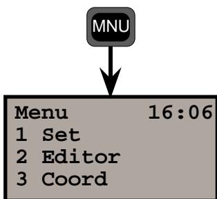
*Turn on the instrument, press the MNU key, the following will be displayed (it is assumed that the compensator has been switched off or that calibration has been made)*
