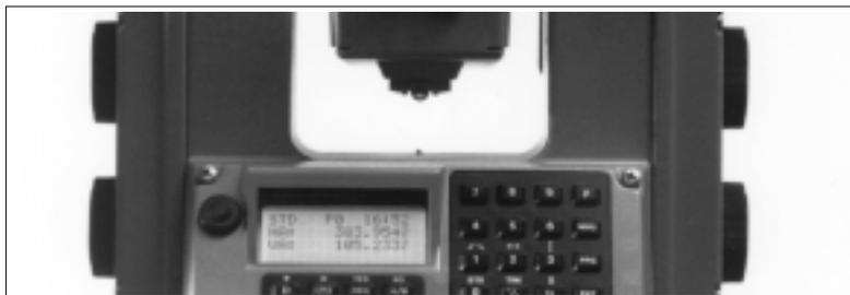
Fig 1.3 Geodimeter Controls (servo instruments)
