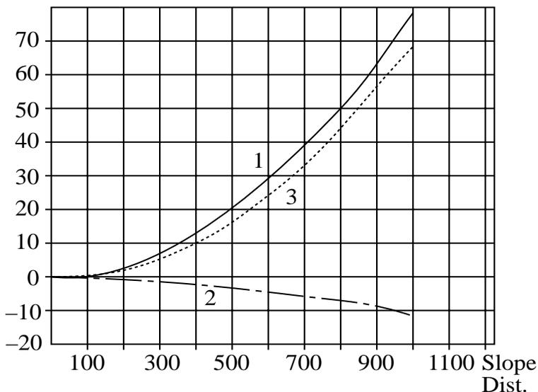
Curve 1 represents the earth's curvature. Curve 2 is the correction for refraction as a function of slope distance. Curve 3 is the resultant correction to be applied to the height obtained by multiplying the slope distance by  $\cos z$ . This correction changes relatively slowly in relation to the deviation from the horizontal plane. At  $20g$  ( $Z=80g$ ), the corrections will have decreased 10%.
