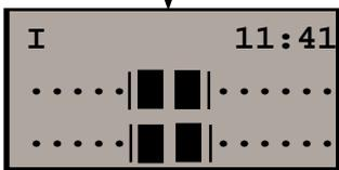
*You now return to the mode that was current before you pressed the function key. The new instrument height is now stored in the instrument.*
