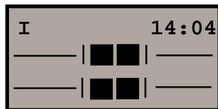
The instrument is levelled.
