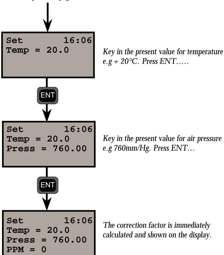
Key in other values for temperature and pressure and see how the ppm changes.
