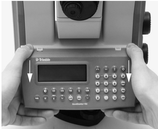
Figure 1.5 How to attach/detach the control unit.
