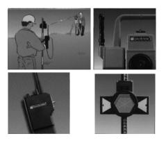
With an instrument, a telemetric link and an ordinary prism you can work with remote surveying which enables you to have the control over the measured data from the point.
