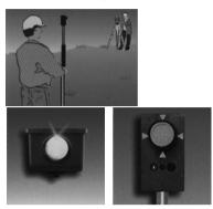
Secondly you can equip your instrument with a tracker unit and take full advantage of the feature we call Autolock<sup>™</sup>, this enables the instrument to lock on to a RMT and automatically follow it as it moves. This means that there is no need for fine adjustment or focusing.
