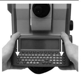
Attaching/Deattaching the Elta CU to the Trimble 5600 Series total station.
