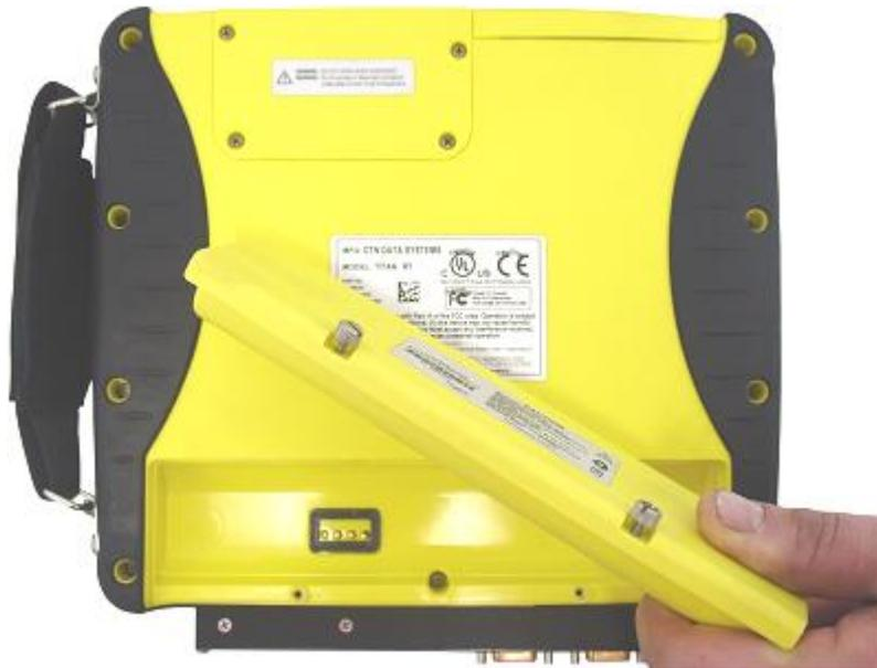
Figure 2. Optional Lithium Ion Battery Pack
