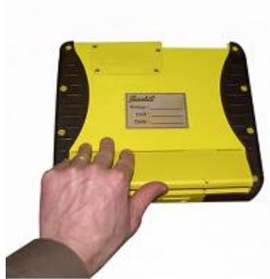
Figure 13. Installing the Optional Battery Pack
