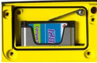
Figure 4. CF Card and Adapter in the Card Slot
