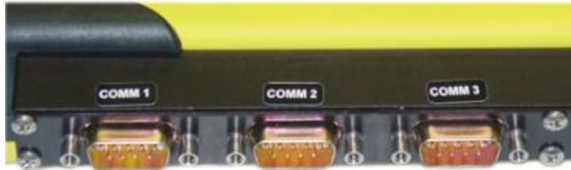
Figure 9. Serial Communication Ports on the Titan RT
