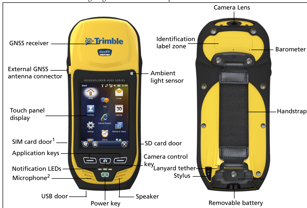
Figure 2.1 Parts of the GeoExplorer 6000 series handheld
